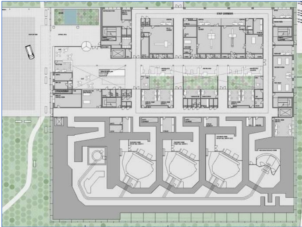
Figure 70: Courtesy Hakan Nyström - Layout of the Danish Center for Particle Therapy (cyclotron and three treatment rooms).
