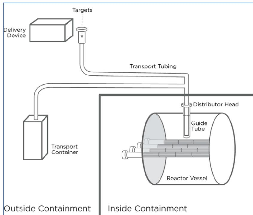
**Figure 34: Principle (simplified) of  $^{177}\text{Lu}$  production in Bruce Unit 7 through vertical guide tube**
