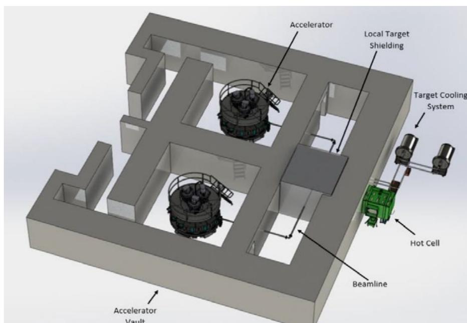
**Figure 33: A twin-Rhodotron® production cell of the NorthStar projected plant<sup>73</sup>**
