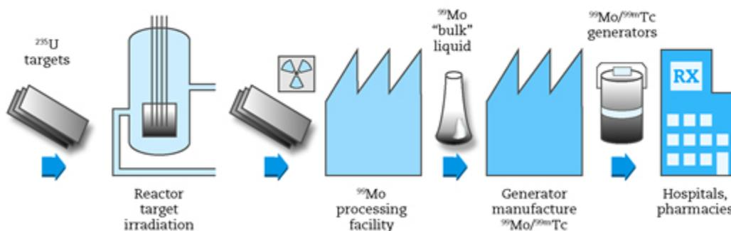
Figure 43:  $^{99}\text{Mo}/^{99\text{m}}\text{Tc}$  supply chain - Source: Ponsard 2010
