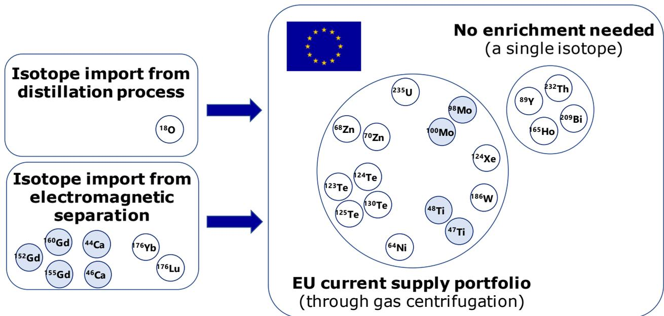
**Figure 12: Current European situation for isotopes enrichment (in blue, isotopes that would be needed by 2030 to support research and/or industrial radionuclide production)**
