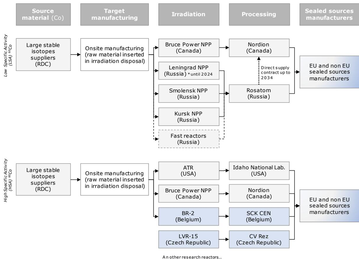
**Figure 64: Current supply chains for  $^{60}\text{Co}$ , for HSA (upper figure) and LSA (lower figure) National production for local markets (India, China) is not included**
