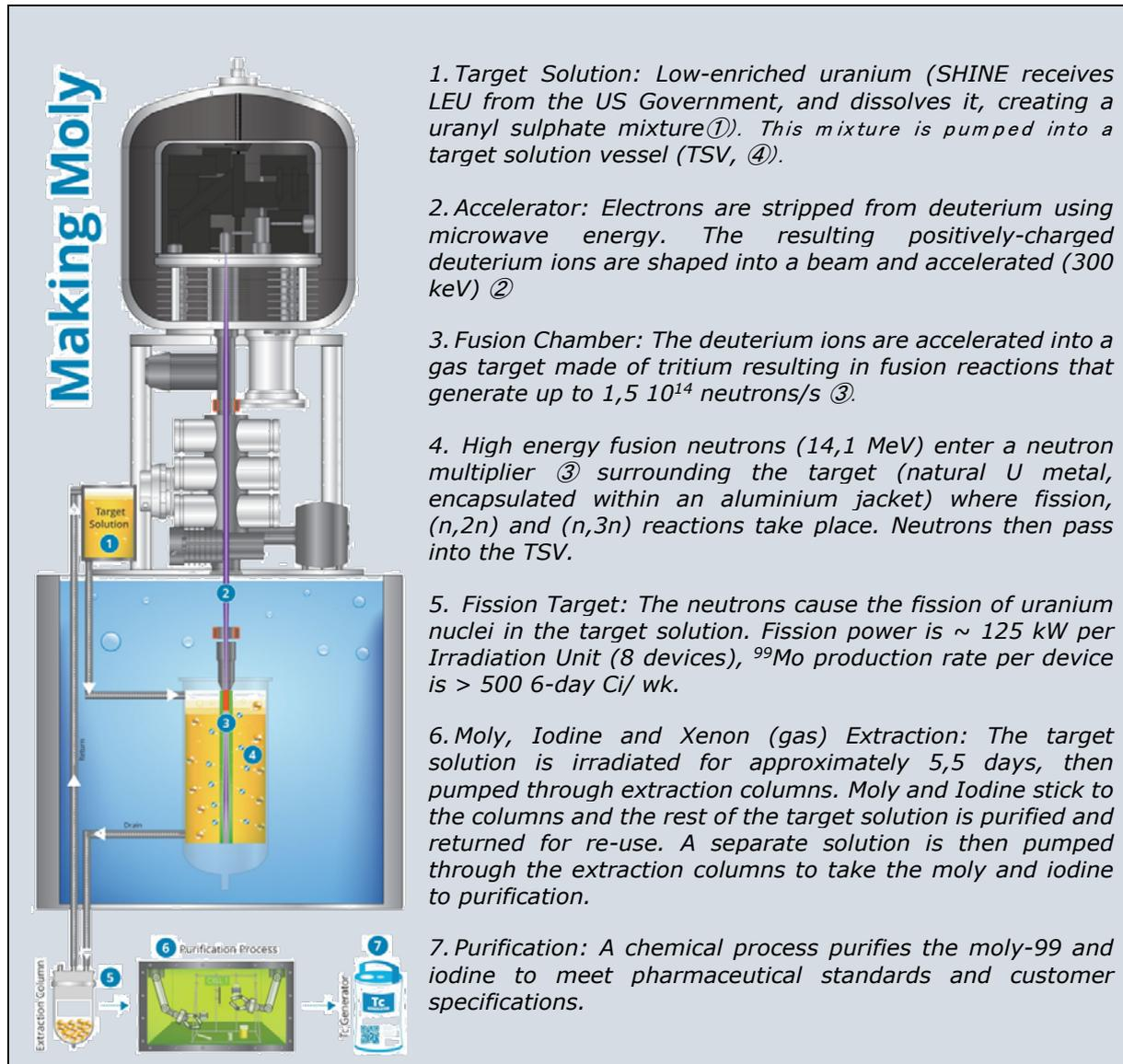
One irradiation unit of the SHINE installation (8 units are foreseen) is illustrated below. The accelerator is connected with the tritium target, inserted in the target solution vessel (not represented). Tritium laboratory is pictured on the left. Other auxiliary systems are not shown. Accelerator + target vessel height is about 8 meters.
