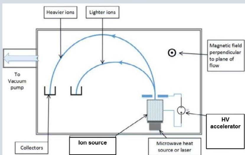
**Figure 15: Calutron principle**
