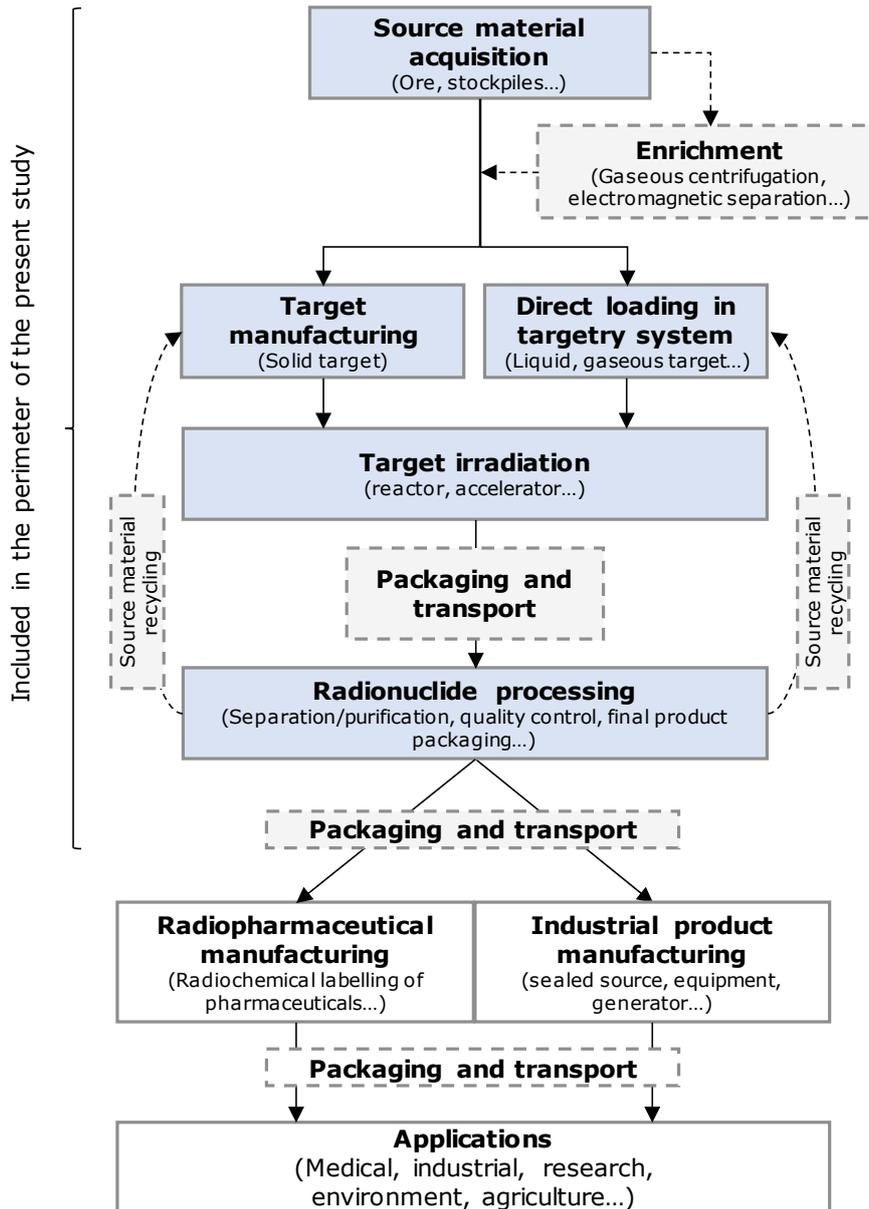
Figure 10: Typical supply-chain steps for radionuclide production
