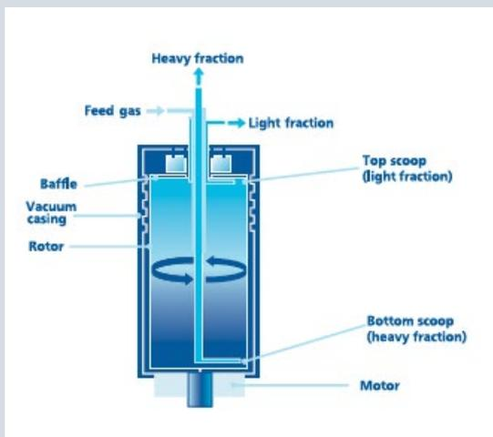
**Figure 14: Principle of a gaseous centrifugation cell centrifuge (Courtesy of Urenco)**
