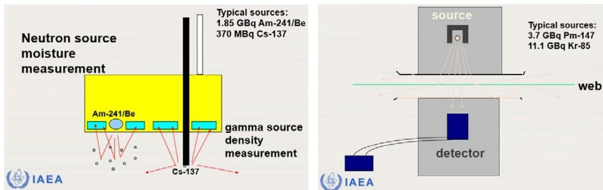
Figure 7: Examples of gauges used in Industry for moisture (Left) and thickness measurement (Right) – Source IAEA
