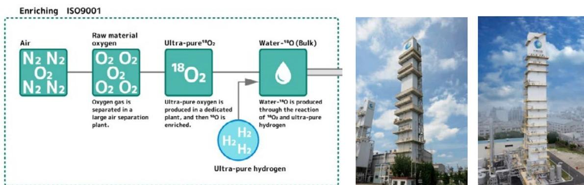
**Figure 16: Front-end of <sup>18</sup>O manufacturing process (packaging and QA not included) and <sup>18</sup>O distillation units 1&2 at Chiba production sites (respectively 100 & 200kg/year). Source: Taiyo Nippon Sanso**
