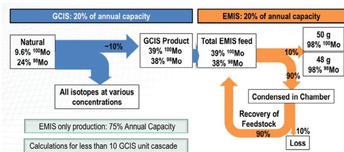
**Figure 18: Production principle for enriched <sup>98</sup>Mo in ESIPP – Source Enriched Stable Isotope Pilot Plant ORNL/DOE**
