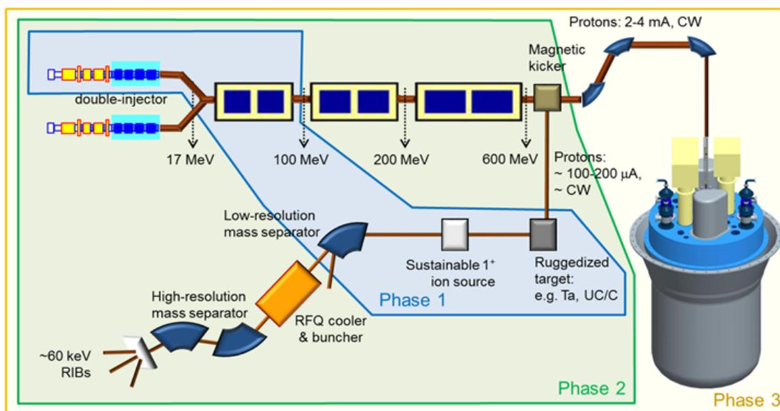
**Figure 30: Myrrha project breakdown into 3 phases and installation principle**
