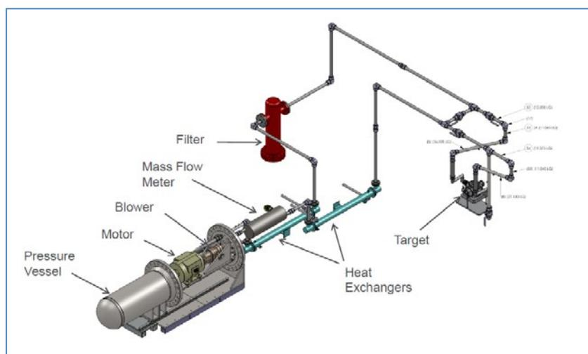
Figure 20: He cooling system for the NorthStar production cell
